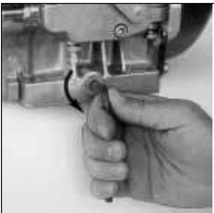
Remove drain plug and drain oil into an approved container. Reinstall drain plug.
