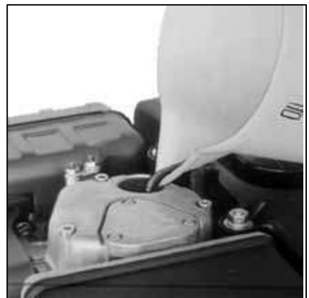
Fill to correct level with oil. Reinstall fill cap
